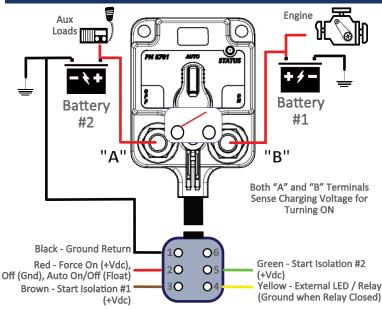
DTM 06-6S Connector End. Customer Supplies DTM04-6P or Cuts & Uses Individual Wire Terminations
